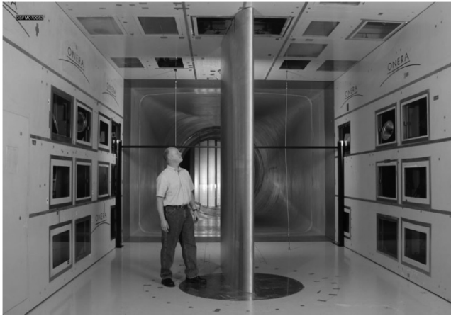
Fig. 1 Photograph of full-scale NACA 23012 airfoil model installed in ONERA F1 wind-tunnel test section.
